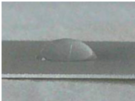
No SOLDERGUARD™ 100 Treatment After 1 hour @ 155°C
