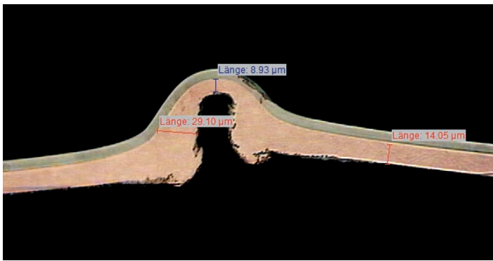
Poor copper throwing power
